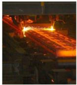
range of 1200°F (650°C). Bearings supporting the pinch rolls were located outside the furnace walls and reached temperatures up to  $750^{\circ}$  F (400°C) due to heat transmitted through the furnace wall by the shaft.
